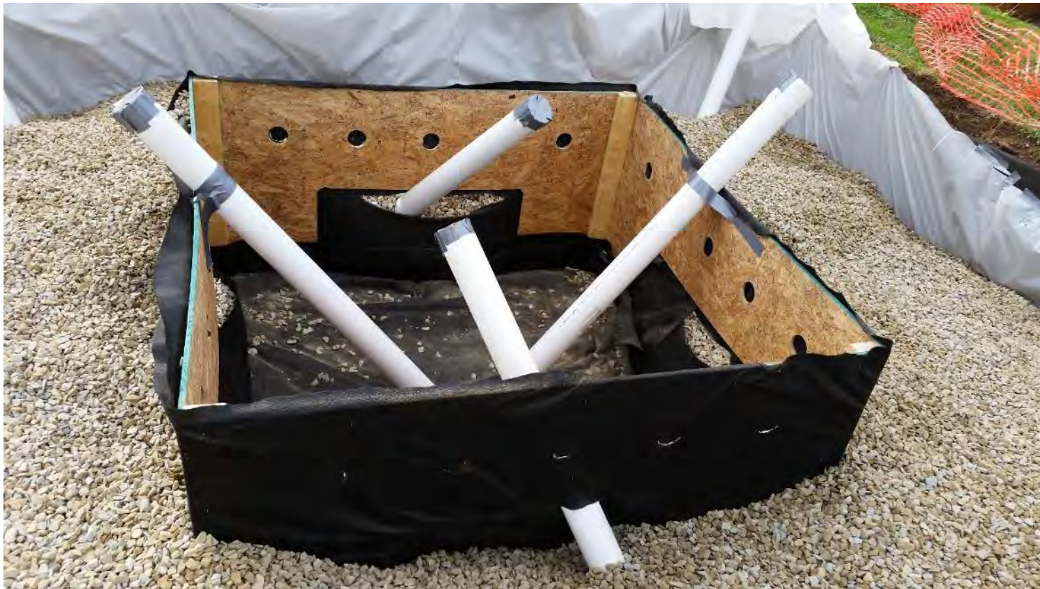
PVC place-holders for clear plastic mini-rhizotrons to observe root growth
