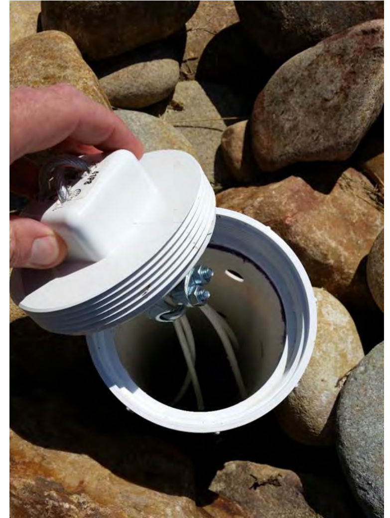
Perforated observation well with HOBO water level data logger
